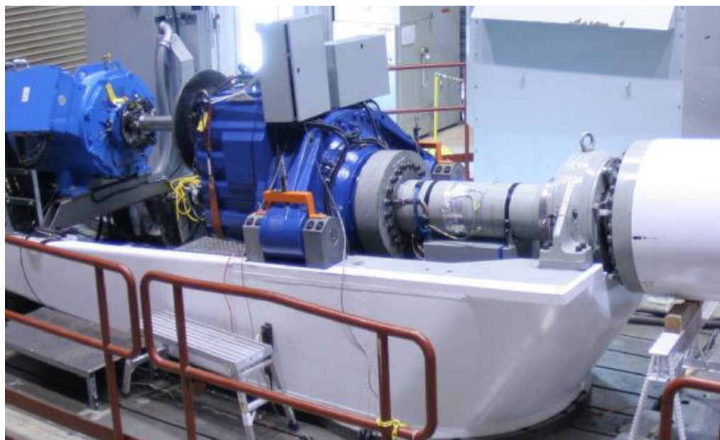
(b) Drivetrain for dynamometer testing [82]
